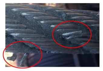
Fig. 5. The detail of the place with two local ruptures of the rope wires
